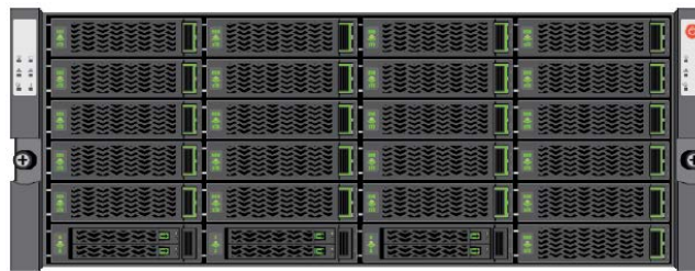
Nimble Storage CS1000 Adaptive Flash Array 6 (Base array, 4U; 21 bays hold carriers with Large Form Factor HDDs, 3 bays hold Dual Flash Carriers with Small Form Factor SSDs)
